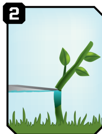
2 WetBlade™ presents herbicide precisely and only at the time of cut, eliminating drift and leaching.
